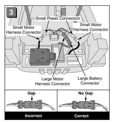
Fit both small motor harness connectors to the small power connectors.
